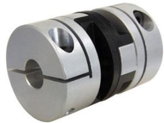
Oldham Couplings: 3000rpm/peak torque 30Nm ( https://www.ondrives.com/bg50-t )
