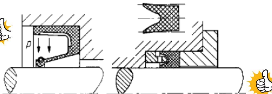
Self-energising in radial lip and U shape seals
